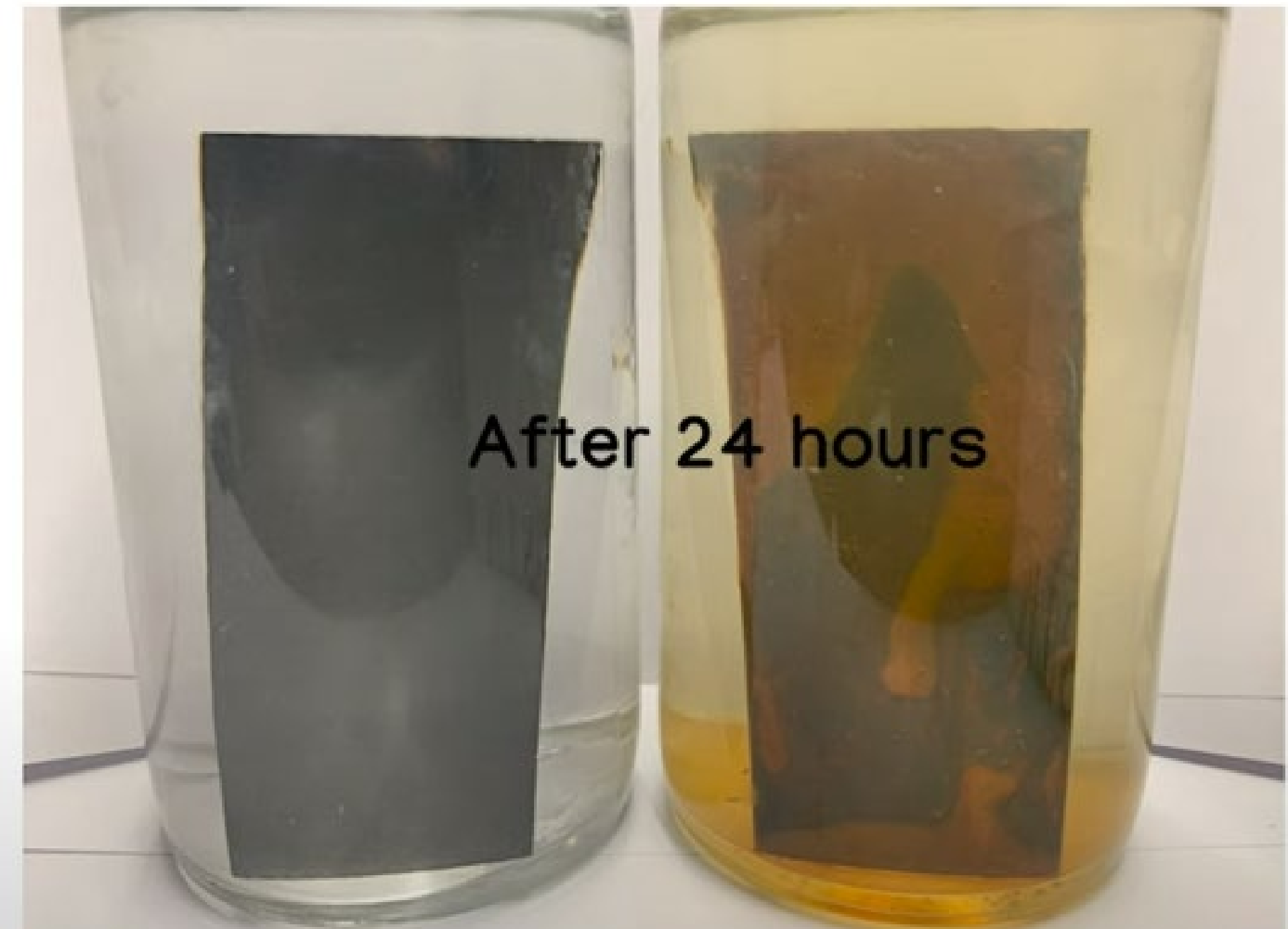
Corrosion Control Treatment Equilibrium Blended Phosphate vs Without
